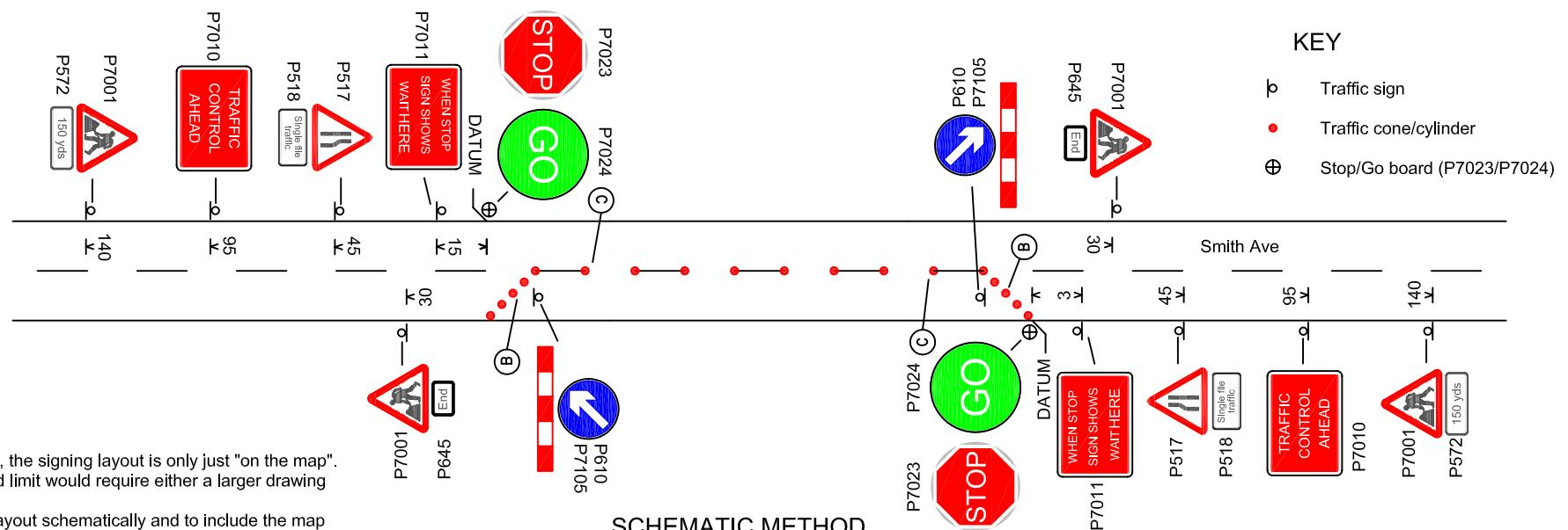
In the to scale example above, the signing layout is only just "on the map". A longer site or a higher speed limit would require either a larger drawing frame or a smaller scale map.
